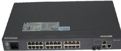
**Fig.2.9** LAN switch Quidway Huawei 3328.
