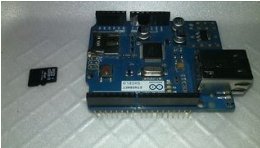
Figura 29 Shield Ethernet y tarjeta microSD
